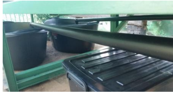
Downward angle of return pipe to the sump
